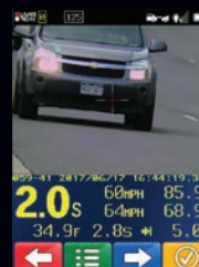
TAILGATING (OPTIONAL) Measure the speed, traveling time and distance between two vehicles.
