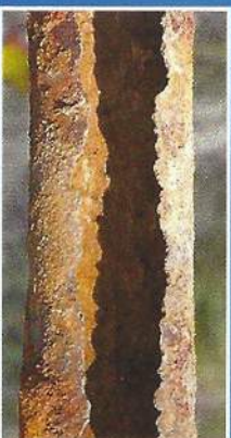
Horizontal Pipe Rot Under Slab
